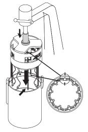
\*Insertion studs must be removed after stators are installed. DO NOT USE INSERTION STUDS in final assembly.
